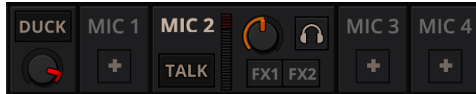
Fig. 1: The microphone ducking controls
