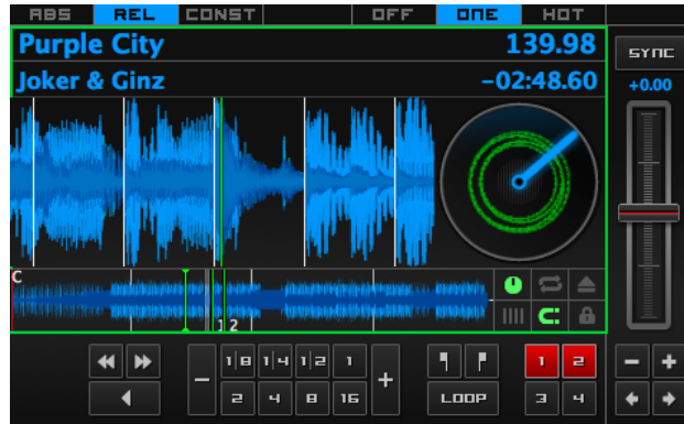
Fig. 5: The vinyl control status, and signal quality display of the deck
